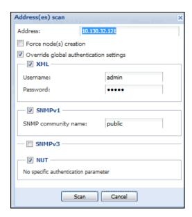
Figure 10. Address(es) Scan Dialog Box (Example 1)
