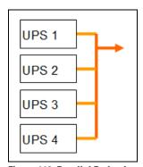
Figure 112. Parallel Redundancy Schema
