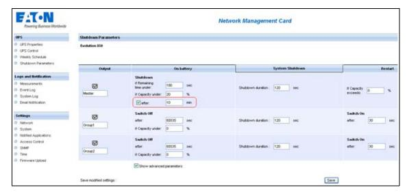
Figure 122. Network Management Card Shutdown Parameters
