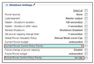
Figure 34. Shutdown Settings-Current Power Default Setting (Priority 5)
