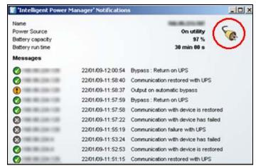
Figure 18. Alarm Notification Box with System Tray Icon
