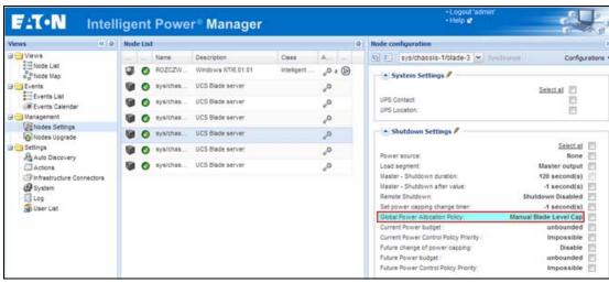
Figure 33. Manual Blade Power Capping
