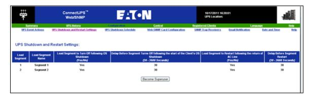
Figure 120. UPS Shutdown and Restart Settings
