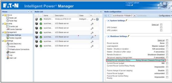
Figure 32. Policy-driven Power Chassis Group Power Capping
