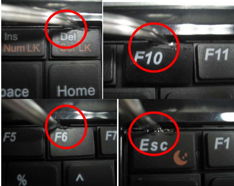
2. After opening the keyboard, remove it as shown below.
