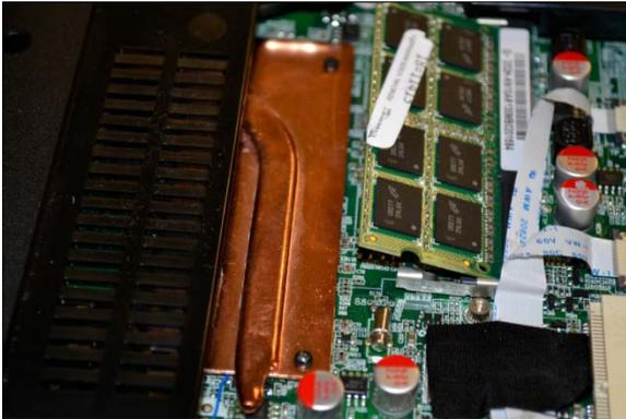
3. Press the memory module down and the metal clip at each side of the DIMM slot will automatically close.
