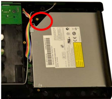
Then detach the Optical Drive cable connector:
