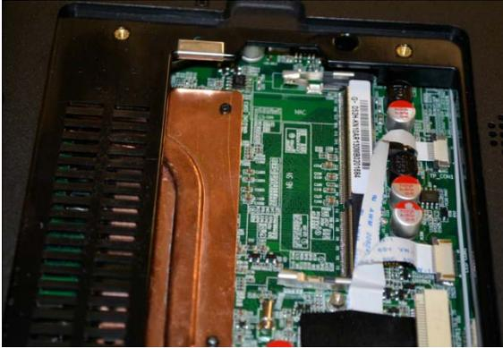
2. Insert the memory module into the DIMM slot at a 45° angle. Then push it in until the golden finger on the memory module is deeply inserted in the DIMM slot.
