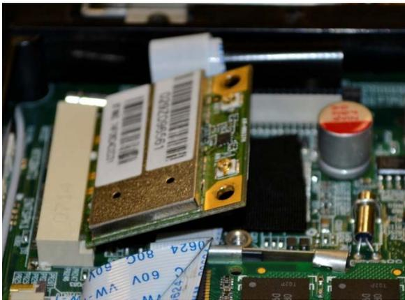
2. Press down the Mini-PCle card and secure the screw to complete the installation.
