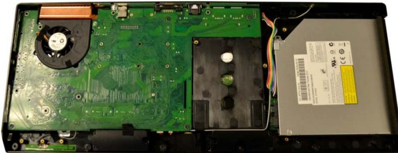
7. Right side-Optical Drive: loosen the cable connector and remove one screw.
