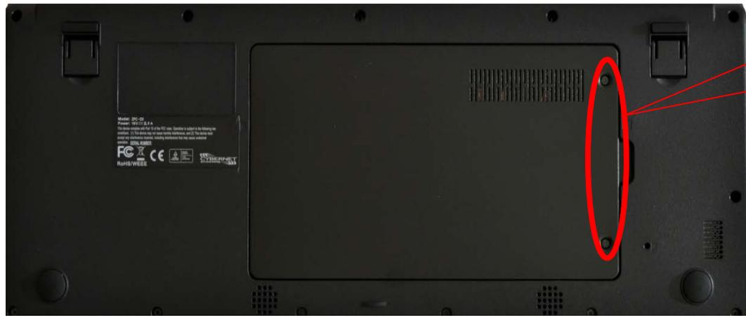
Loosen two screws to remove cover.
