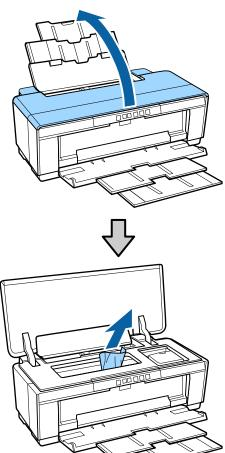
After removing the paper, close the printer cover and press the D button to cancel the error.
