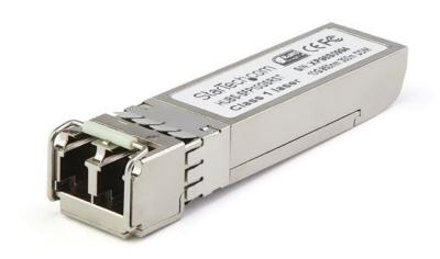
The SFP10GZREMST is a Dell EMC SFP-10G-ZR compatible fiber transceiver module that has been designed, programmed and tested to work with Dell EMC brand switches and routers. It delivers dependable 10 GbE connectivity over fiber cable, for 10GBase-ZR compliant networks, with a maximum distance of up to 80 km (49.7 mi).
