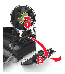
Press the green levers on each side of the waste toner bottle, and then remove the waste toner bottle.
