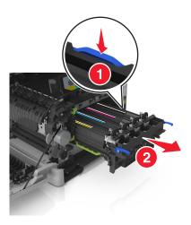
**8** Remove the used developer unit.
