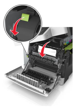
**4** Hold down the fuser cover, and then remove the jammed paper.
