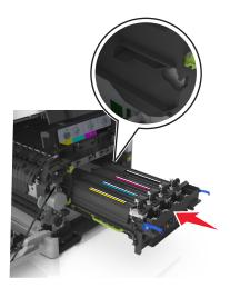
15 Gently but firmly push the blue levers down until the imaging kit fits into place.
