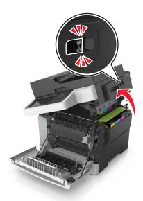
Remove the toner cartridges by lifting the handles, and then gently pulling them away from the imaging kit.
