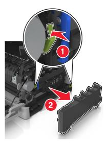
Lift the blue levers on the imaging kit, and then pull the imaging kit until it stops.
