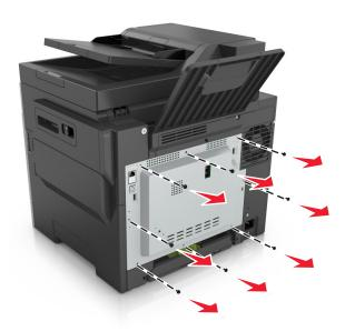
2 Slightly open the controller board access cover, and then shift to the right to remove it.
