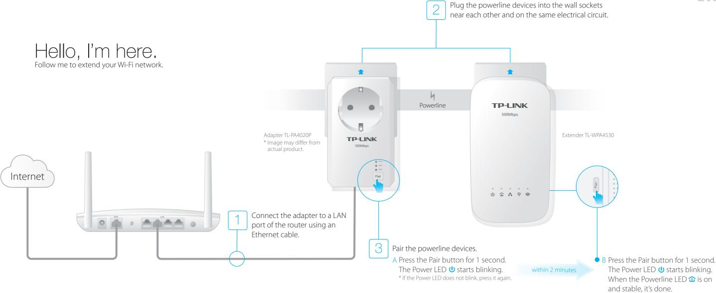
Find the Wi-Fi Info Card in the package, and then relocate the powerline extender to a new location. Connect to the Wi-Fi using the SSID and password on the card.
