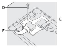
6. Pull out the built-in bridge battery with the sheet cover.
