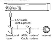
The use of a shielded and straight interface cable (LAN cable) is recommended
