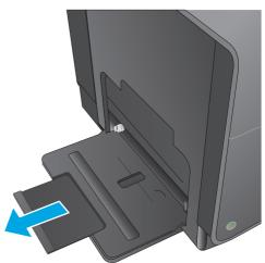
3. Extend the paper guides fully and then load the paper stack into Tray 1. Adjust the paper guides to the size of the paper.
