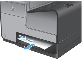
3. If the jammed sheet is not visible or easily accessible in Tray 1, open the left door to access the jammed sheet.
