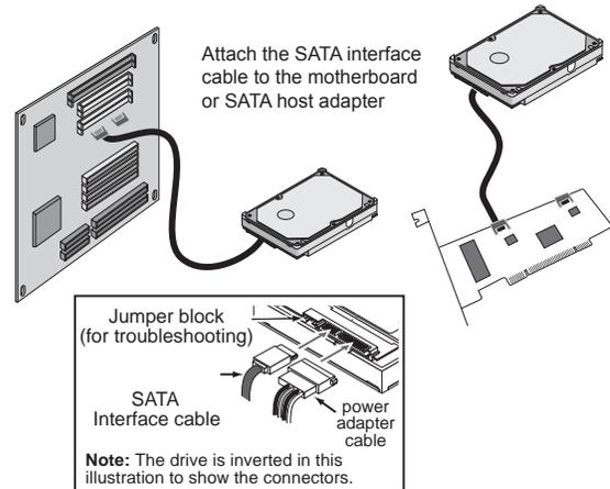
**Note.** Serial ATA connectors are keyed to ensure correct orientation.
