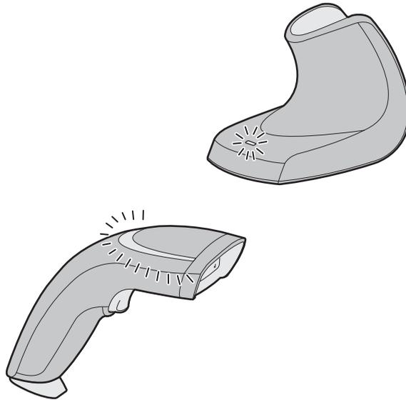
**Bluetooth Connected—Intermec-Ready-to-Work Indicator On**
