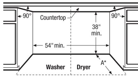
**Side-by-Side Units in Under-Counter Installation**
