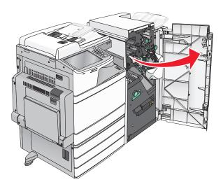
**2** Press the latch to open the stapler door.
