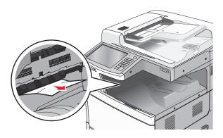
1 Open door A, and then door D by lifting the release latch of each door and lowering the doors.
