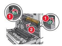
3 Lift the green lever, firmly grasp the paper on each side, and then gently pull it out.
