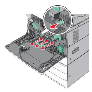
Slide the printhead wipers back into place.
