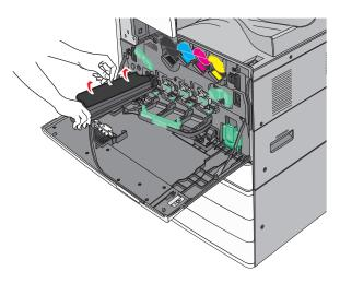
Push the tab forward to insert the photoconductor unit.
