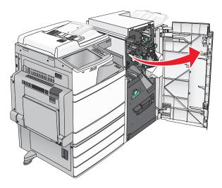
**2** Grasp the handle of the staple cartridge holder, and then pull out the holder to the right.
