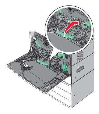
**7** Slide the release lever to the right to lock the cover.
