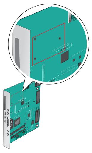
**Note:** If an optional ISP is currently installed, then the printer hard disk must be installed onto the ISP. To install a printer hard disk onto the ISP:
