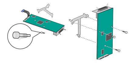
Use the provided screw to attach the ISP solution to the system board cage.
