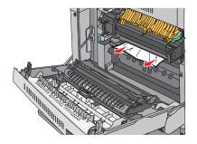
**b** If the paper is not visible, then you will need to remove the fuser unit.
