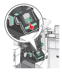
**4** Squeeze both sides of the empty staple case with your fingers, and then remove the staple case from the cartridge.
