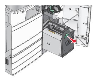
**8** Lift the inside cover. If the paper is jammed in the rollers, then rotate knob G8 counterclockwise, and then remove the jammed paper.
