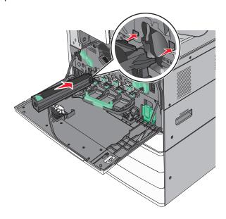
Remove the tape from the top of the photoconductor unit.
