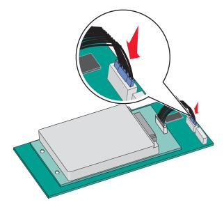
To install a printer hard disk directly on the system board:
