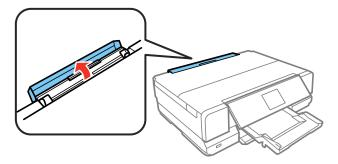
3. Fully extend the paper support and tilt it back, as shown.
