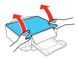
2. Place your original facedown on the scanner glass with the top of the original facing into the corner shown. Slide the original to the edges of the indicated corner.
