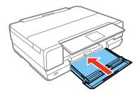
**Note:** The output tray opens automatically when you print. Leave enough space in front of the product for the paper to be fully ejected. Do not remove or insert the paper cassette while the product is operating.
