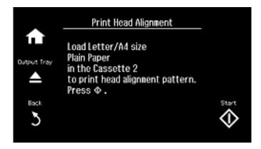
7. Press the **Start** button to print an alignment sheet.
