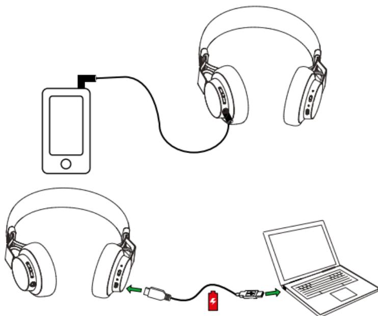
**NOTE:** Bluetooth connections are disabled when connected to the 3.5 mm Jack Connector.
