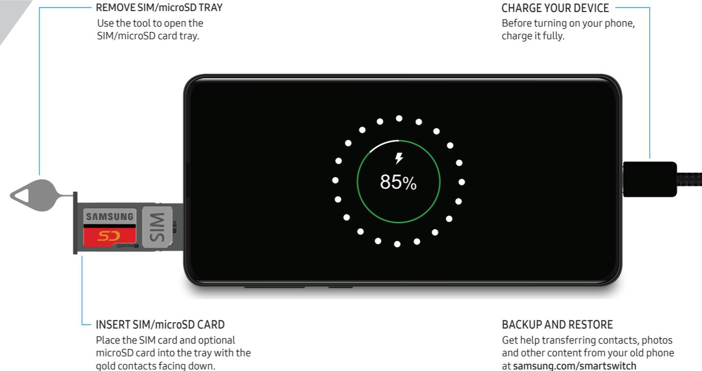
Note: Use only Samsung-approved charging devices and accessories. Samsung accessories are designed for your device to maximize battery life. Using other accessories may void your warranty and may cause damage.
