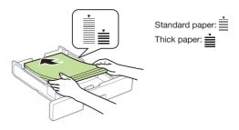
**Note:** Make sure the paper is under the arrow mark for your paper type and loaded against the front edge of the cassette.
