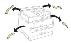
**2** Lift up the scanner unit and remove all protective materials from inside the product, then close the scanner unit.
