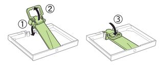
**Note:** Make sure the ink pack is fully inserted and level with the top of the ink pack tray.
