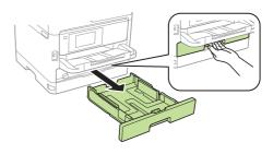
**2** Slide the side edge guides all the way out and set the front edge guide to the paper size you are using.
