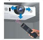
The intuitive motorised vertical and horizontal lens shift mechanism provides fast and efficient installation. This allows users to easily adjust images up to ±50% horizontally and up to 70% vertically, depending on the models and lenses used. This functionality is ideal for theatres and conference suites that require continuous changes to projection set-ups. Each model features a two speed motorised lens for focus, zoom and lens shift.
