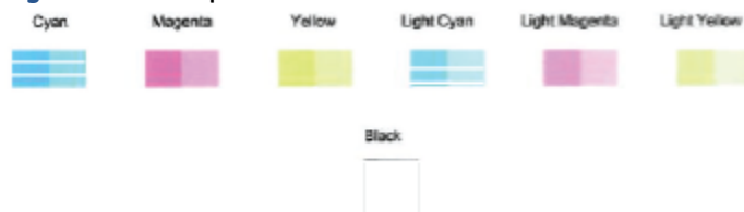
Figure 9-2 Example of color blocks with defects
