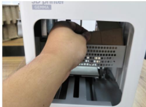
Insert the Filament Guide Tube into the pneumatic connector on top of the Extruder.
