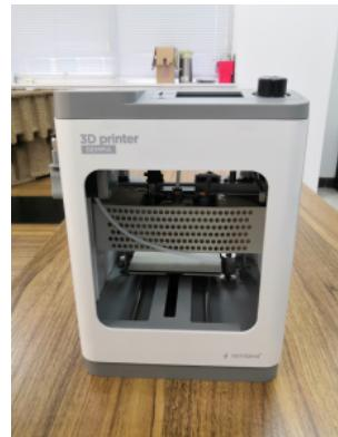
Remove the carton block in the printer.
