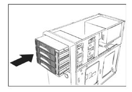
Using the mounting screws provided, secure the Multi-Drive Enclosure to the drive bays:
