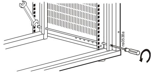
2. Remove the rods from the enclosure.
