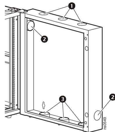
For unrestricted access to the back of the enclosure when the standard openings are insufficient, remove the six screws securing the access plate to the bottom of the rear door.
