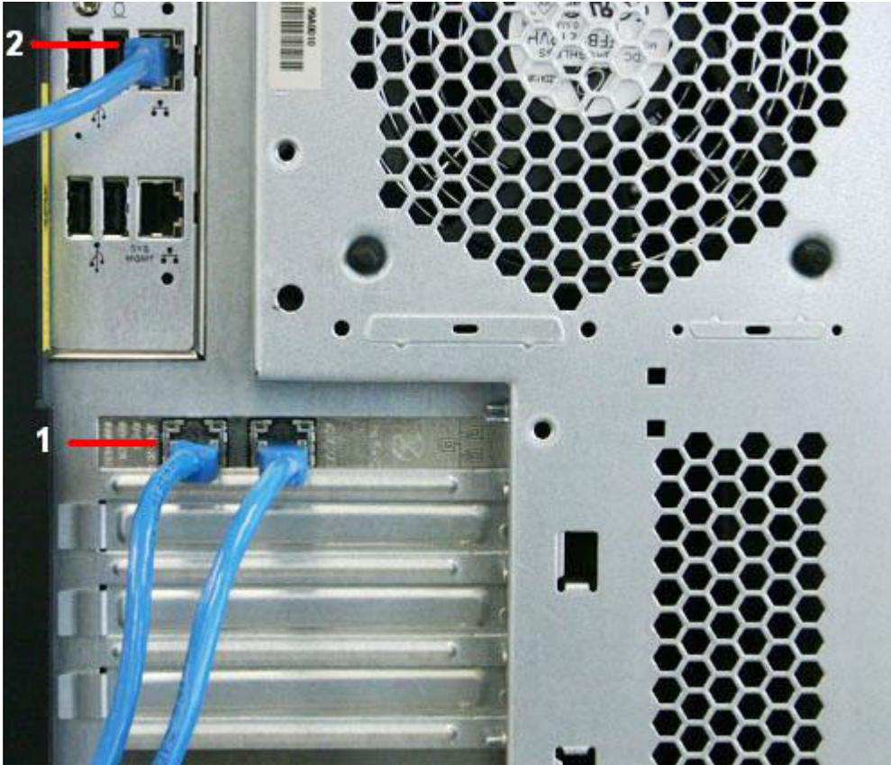
Figure 1. View of Ethernet ports 1 and 2
