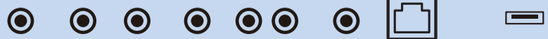
RS232 IN RS232 OUT IR-IN IR-OUT AUDIO OUT PC LINE IN RJ45 USB 2.0 5V/0.5A
