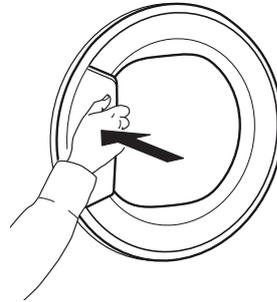
If you interrupt a running programme by opening the door, the programme will be reset if the dryer door is not closed again within one minute.
