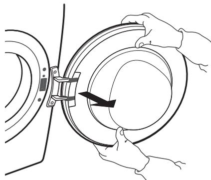
**5.** Fix the door on the left side by turning in the 2 screws. Take care to screw them in vertically, to avoid pinching off the door seal.
