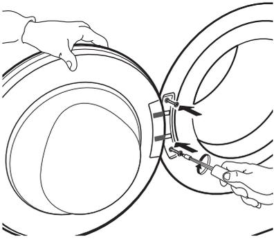
**6.** Insert the door lock on the right side of the door opening. Press it completely inside the hole and move it a bit downwards, until the small knob of the door lock latches.
