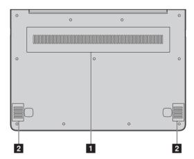
**1 Ventilation slots** Dissipate internal heat.
