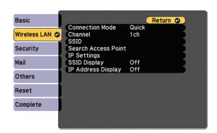
4 Choose **Connection Mode**, press \(\frac{4}{\Omega}\), select **Quick** for a direct connection to a computer, tablet, or smartphone, then press \(\frac{4}{\Omega}\) again. When you're finished, press **Esc** to return to the Wireless LAN menu.
