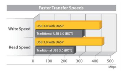
At the same peak in testing UASP also shows an 80% reduction in required processor resources.
