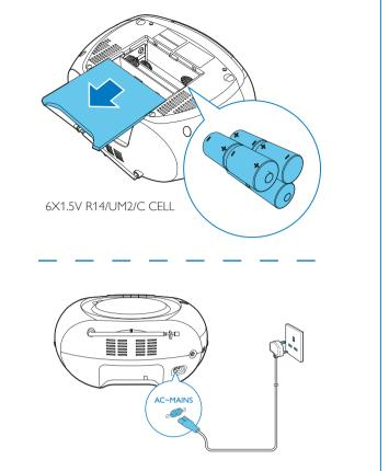
To play with the device, you can use either alkaline battery (R14) or AC power.
