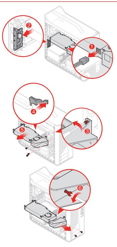
**NOTE:** When you install the PCI express adapter, place the PCI port area toward the EMI gasket with the correct orientation.
