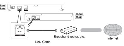
Use category 5 or above straight LAN cables (STP) when connecting to peripheral devices.
