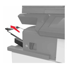
2 Press the latch and slide the staple finisher to the left, and then remove the jammed paper.
