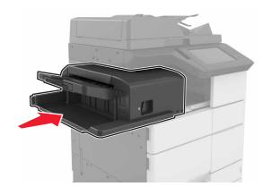
4 Open door C, and then remove the jammed paper.
