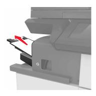
**2** Press the latch on the staple finisher, and then slide the finisher to the left.
