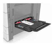
Warning—Potential Damage: Never use envelopes with stamps, clasps, snaps, windows, coated linings, or self-stick adhesives. These envelopes may severely damage the
