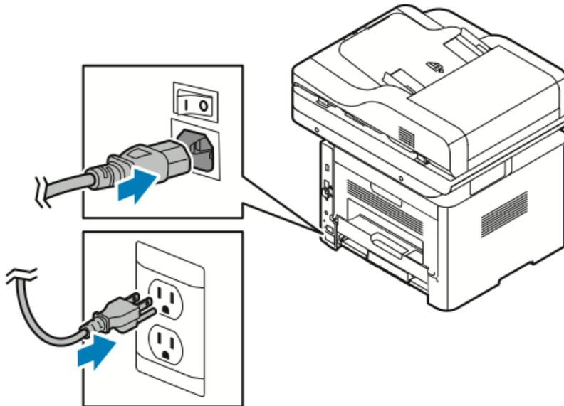
The printer has a *power Down* button on the touch screen and a *power switch* on the back-left side.
