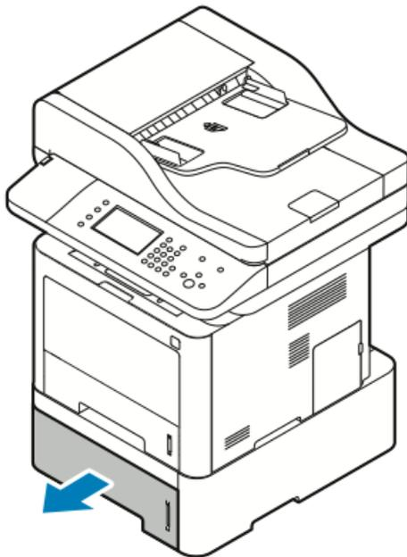
2. To remove any jammed paper, gently pull it straight out as shown.
