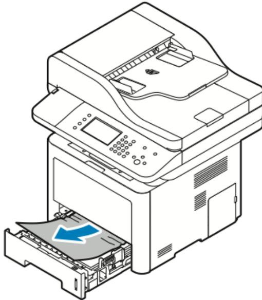
If the paper does not move when you pull it, or if you do not see the paper in this area, refer to [Clearing Paper Jams from the Inside the Printer](#).
