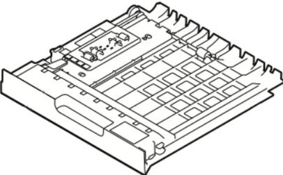
3. Insert the duplex unit back into the printer and push it in all the way.
