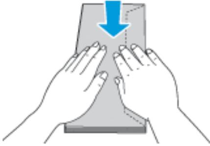
3. To load envelopes, place the envelopes with the print side up, flaps closed and down, and the flap of the envelope to the left.
