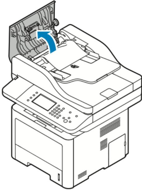
3. If the paper is jammed in the exit of the document feeder, gently pull it out in the direction shown.
