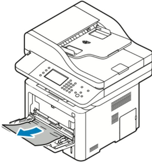
3. If the paper is torn, check inside the printer for pieces of paper, then gently remove them. If you cannot remove the paper fragments easily, contact your Xerox representative.
