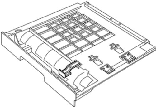
b) Adjust the width guide to match the width of paper you will be using.
