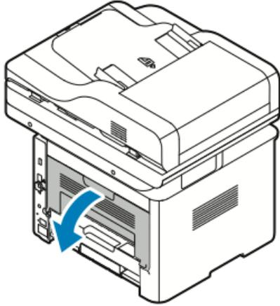
3. Gently remove any jammed paper from the back of the printer.
