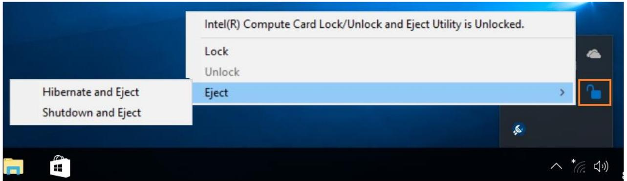
After selecting the eject option, the fan in the Dock will cool the Card to a safe temperature level before ejecting it.
