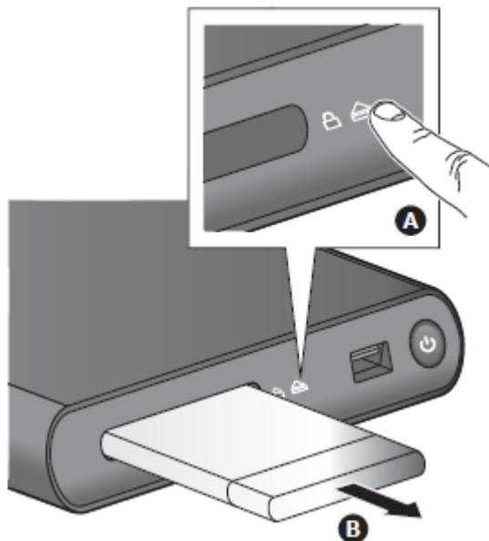
After pressing the eject button, the fan in the Dock will cool the Card to a safe temperature level before ejecting it.
