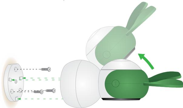
2. Align the wall plate with the holes on the base of the camera and rotate the base until it snaps into place.
