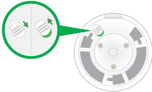
To avoid draining the battery, switch the battery off if you are not using it or if you are moving the camera to a new location.
