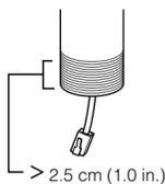
Pass necessary cables for connecting the camera through the pipe.
