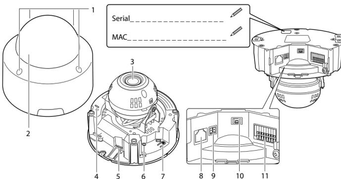
1. Dome case lock screw / 2. Dome case / 3. Lens unit / 4. LED /
