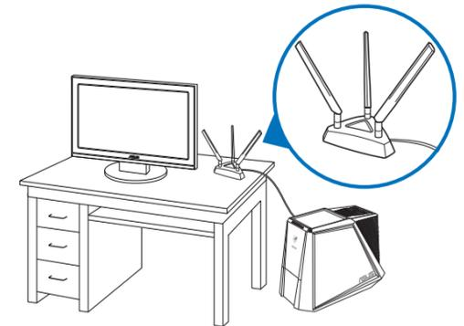
Adjust the magnetic antenna base to get the best signal with your router.
