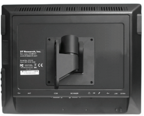
3. Attach the new VESA-compliant mounting device or stand to the display.
