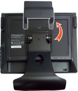
1. Remove the detachable base by pressing upward to remove the cover, then unscrewing the four screws attaching the base to the display.
