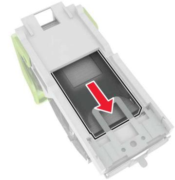
**Note:** If the staples are at the rear of the cartridge, then shake the cartridge downward to bring the staples near the metal bracket.
