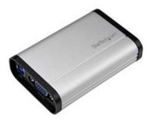
This capture device turns your USB 3.0 computer into a digital video recorder for high-quality VGA video, leveraging USB 3.0 transfer speed to capture raw 1080p video at 60 frames per second. The capture device records video from your VGA source device and also includes a 3.5 mm audio input jack, which lets you record the video's accompanying analog audio output, or add your own independent audio source for voice over commentary.
