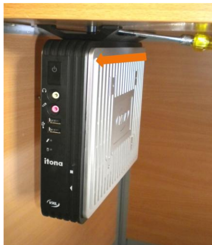
Figure 2-14: Removing the Client
