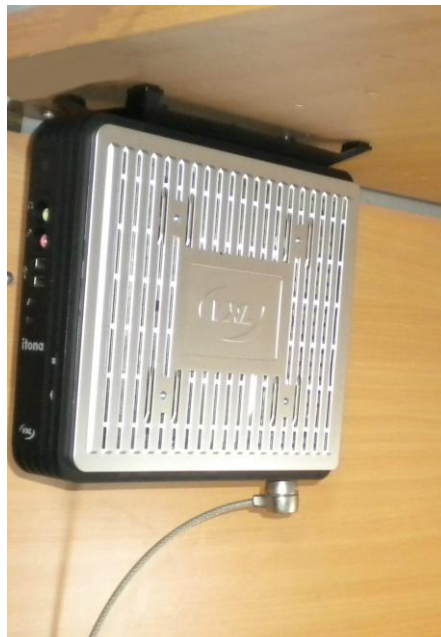
Figure 2-17: Kensington Lock Slot on the Bottom Strip
