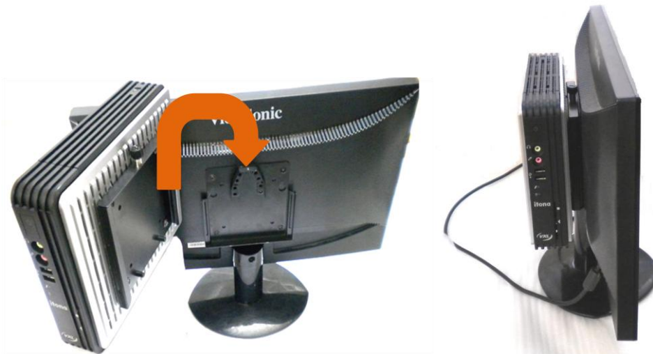
Figure 2-8: Mounting the Thin Client using a VESA
