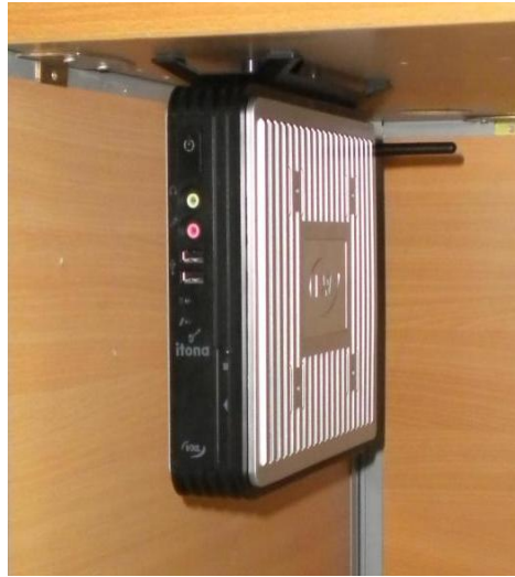
Figure 2-13: Mounting under the Counter Top
