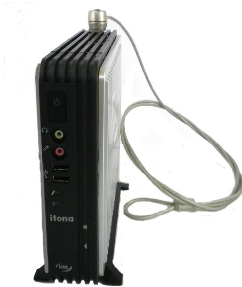
Figure 2-16: Kensington Lock Slot on the Top Strip
