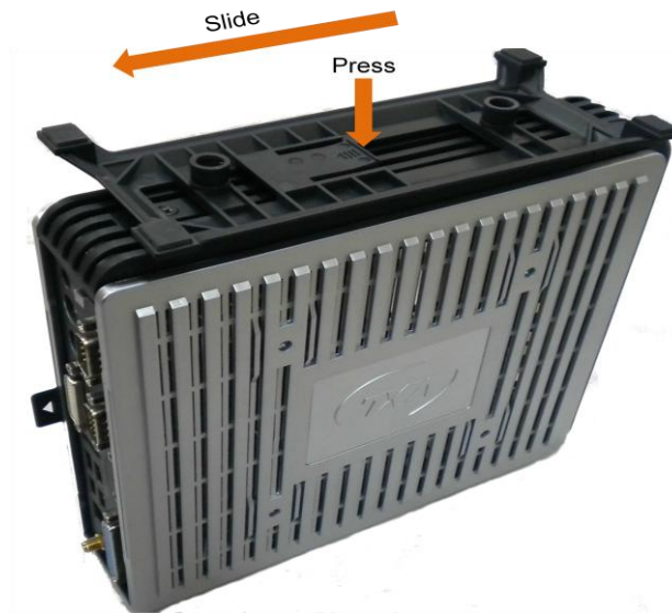
Figure 2-5: Removing the Pedestal
