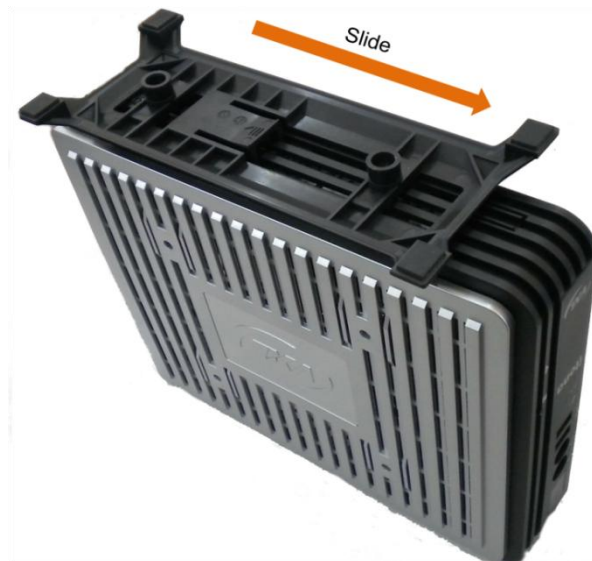
Figure 2-4: Installing the Pedestal
