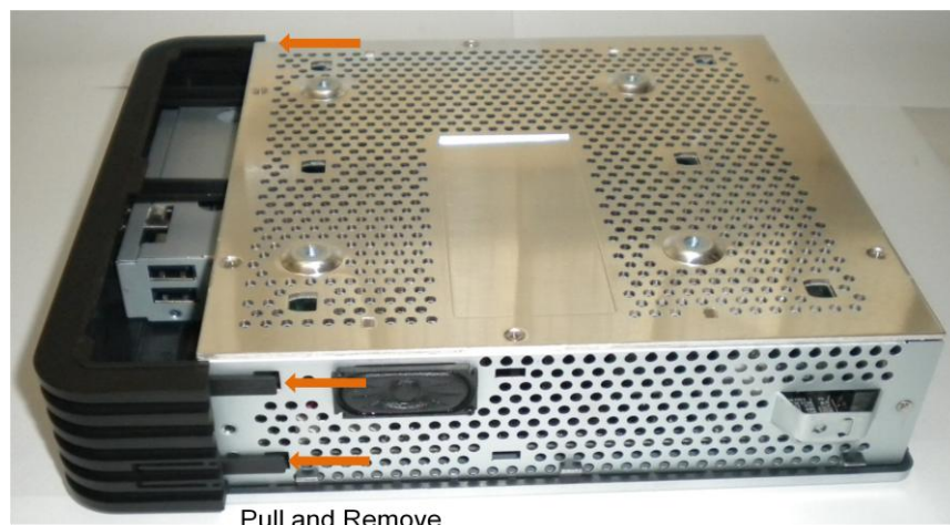
Figure 2-2: Removing the Front Bezel
