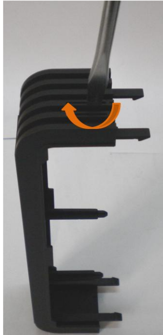
Figure 2-3: Opening the Secure Shell USB Wire Seal
