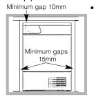
If you are going to install the appliance under a work counter, be sure to leave a 10mm space between the top and any other objects on or above the machine and a 15mm space between
