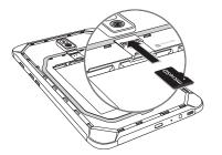
3. Insert the battery, making sure to align the gold contacts and press down.
