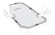
Caution: Devices with accessible compartments or ports should be sealed or closed tightly to prevent liquid from entering the device.
