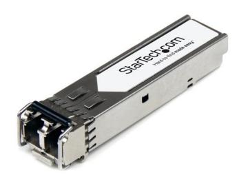
The J9153D-ST is an HP JD093Bcompatible fiber transceiver module that has been designed, programmed and tested to work with HP brand switches and routers. It delivers dependable 10 GbE connectivity over fiber cable, for 10GBase-ER compliant networks, with a maximum distance of up to 40 km (24.8 mi).
