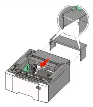
4 Align the printer with the 650-sheet duo drawer, and then lower the printer into place.
