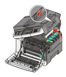
Remove the toner cartridges by lifting the handles, and then gently pulling away from the imaging kit.
