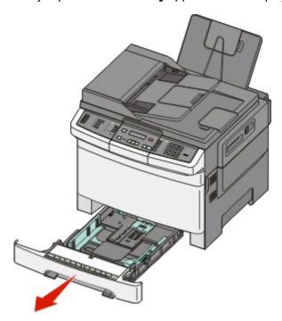
**2** Squeeze the length guide tab inward as shown, and slide the guide to the correct position for the paper size being loaded.
