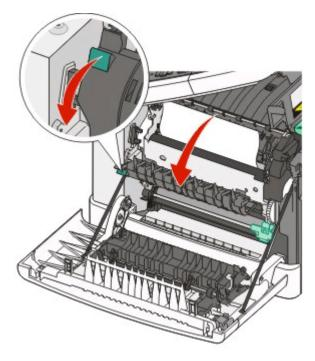
Hold the fuser cover down, and then remove the jammed paper. The fuser cover closes when released.
