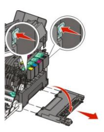
Press the green levers on each side of the waste toner bottle, and then remove it.
