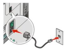
**3** Remove the protective plug from the EXT port **a** of the printer.
