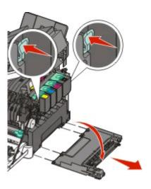
Press the green levers on each side of the waste toner bottle, and remove it.
