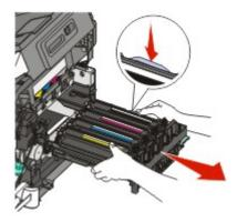
**8** Remove the used developer unit.
