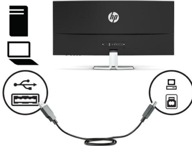
**NOTE:** You must connect the USB Type-B upstream cable from the source device (computer) to the rear of the monitor to enable the USB Type-A downstream ports on the monitor. For more information, see [Connecting USB devices on page 8](#).
