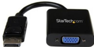
The DP2VGA3 DisplayPort 1.2 to VGA adapter lets you connect your DisplayPort-equipped desktop or laptop computer to a VGA monitor or projector, eliminating the expense of upgrading to a DisplayPort 1.2-capable display.
