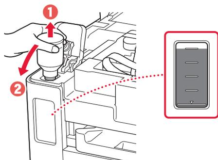
7 Replace the tank cap **securely**.
