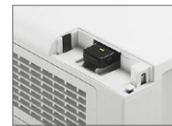
The wireless module ET-WM200U mounted on the projector
