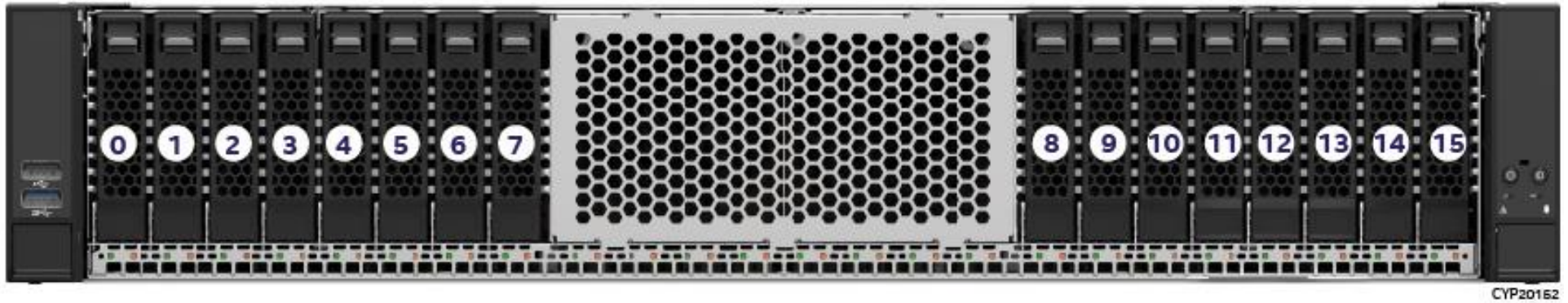
Figure 25. 2U 16 x 2.5" Front Drive Bay Configuration
